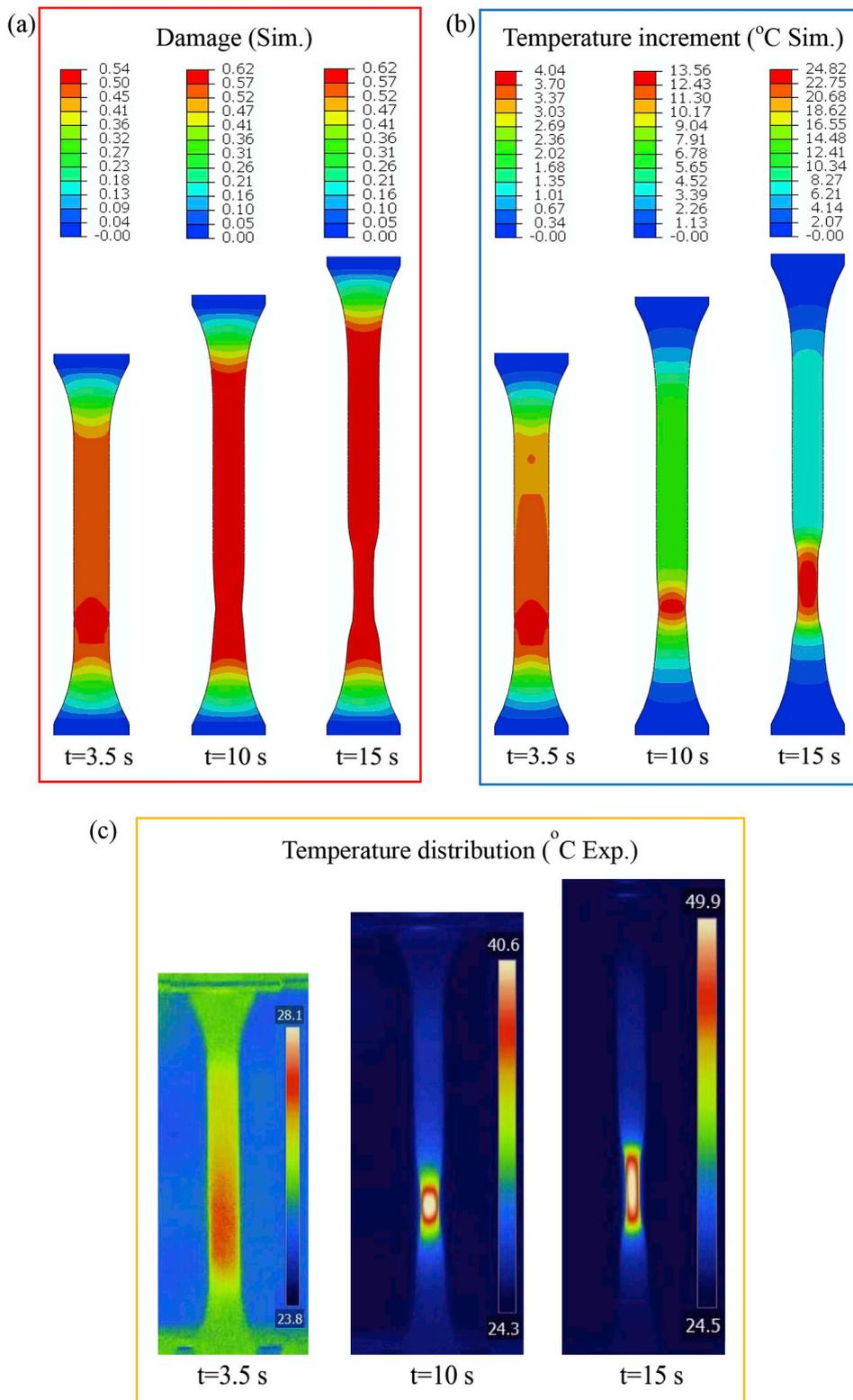
Fig. 8. Distributions of (a) predicted damage, (b) predicted temperature increment and (c) measured temperature on the specimen surface at 3.5, 10 and 15 s.
