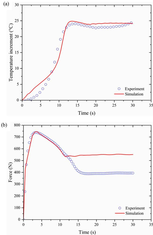
**Fig. 6.** In terms of deformation time for polyamide 6 at 120 mm/min loading rate and room temperature, experimental and numerical results of the evolution of (a) the increment of maximum temperature and (b) the tensile force.
