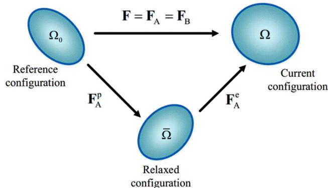
Fig. 2. Schematic representation of deformation gradients in three configurations.
