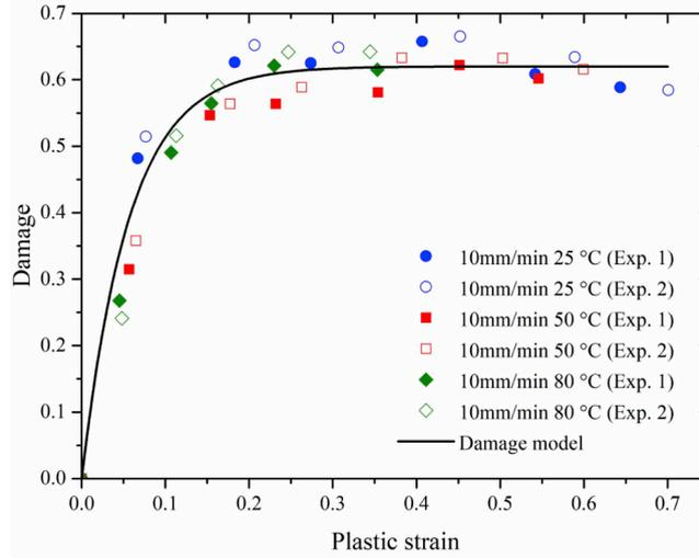
Fig. 5. Experimental and model results of damage evolution of polyamide 6 under 10 mm/min loading rate at three different temperatures.
