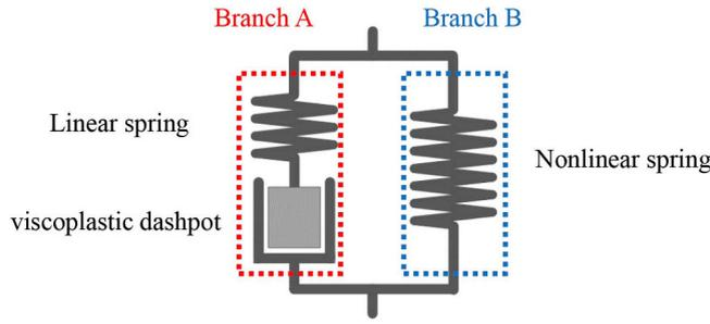
Fig. 1. Schematic of the constitutive model with three elements.
