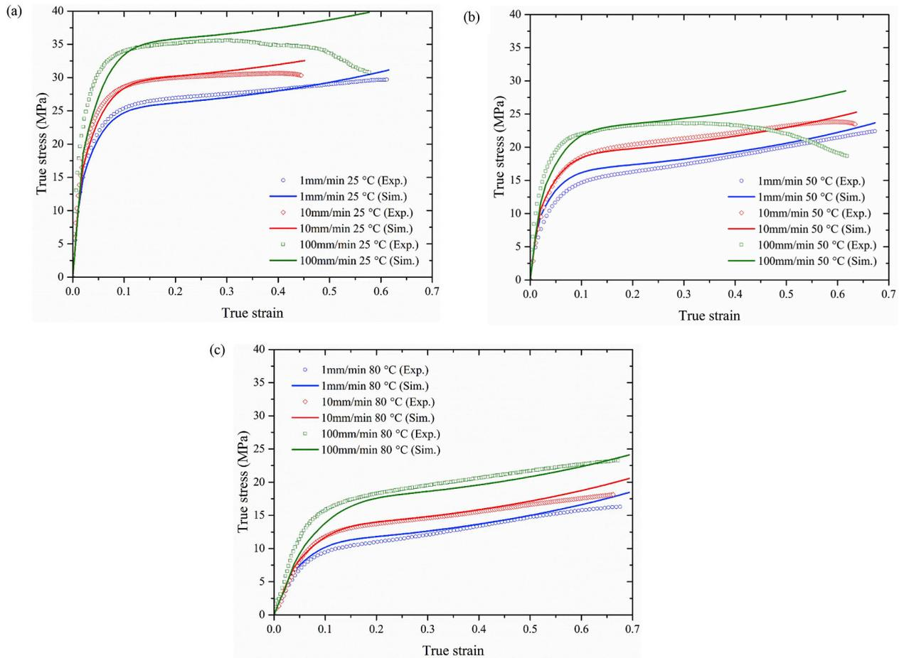
**Fig. 3.** Experimental and numerical results of strain-strain curves of polyamide 6 under three loading rates (1, 10 and 100 mm/min) at three temperatures: (a) 25, (b) 50 and (c) 80 °C.
