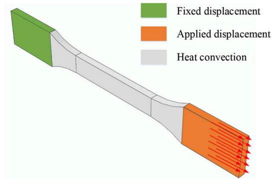
**Fig. 7.** Mechanical and thermal boundary conditions on the specimen.
