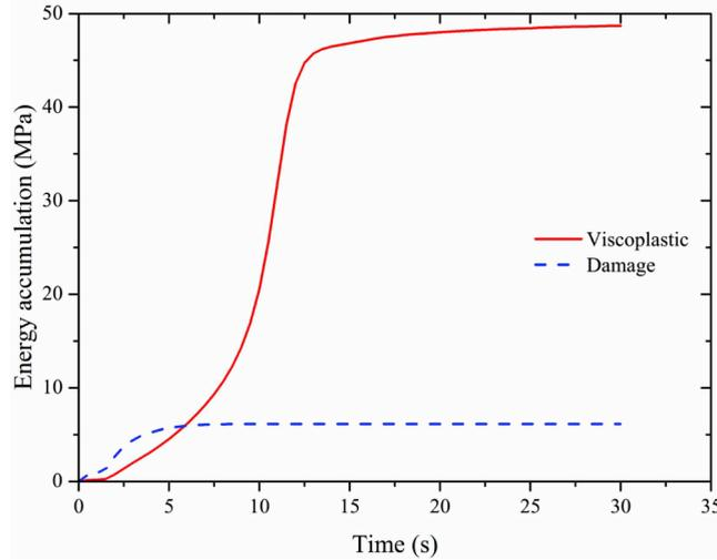
Fig. 9. Evolutions of the viscoplastic and damage energy accumulation with respect to time for a material point in the necking section.
