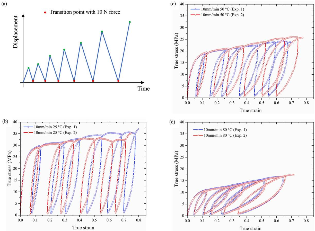
Fig. 4. (a) Schematic of applied displacement history in repeated loading tests. Stress-strain curves of polyamide 6 under 10 mm/min loading rate at three temperatures: (b) 25, (c) 50 and (d) 80 °C.
